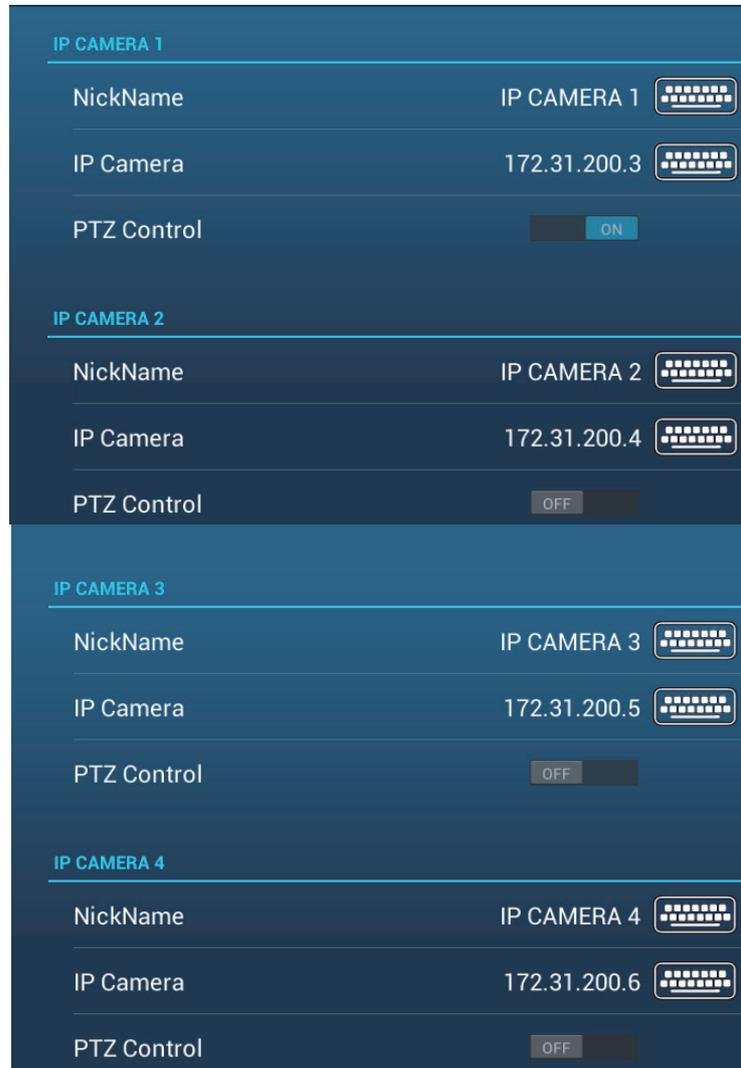
**Nickname:** If desired you can change the name of the IP camera(s). The default names are [IP CAMERA 1], [IP CAMERA 2], [IP CAMERA 3], [IP CAMERA 4]. You can use a maximum of 20 characters. To change a name, tap [NickName] to show the software keyboard. Change the name, then tap ✓ to finish. The name is reflected to the following locations.
