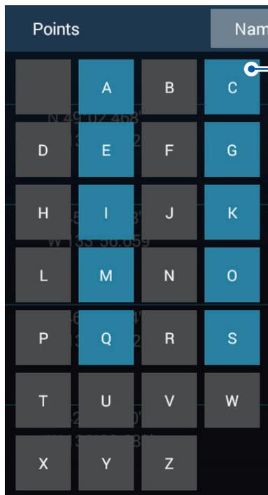
Points which start with a particular letter have the first letter highlighted in the search options. In this example, the points list has points which start with the letter highlighted in blue. Grayed out letters indicate that no saved point names begin with that letter.
