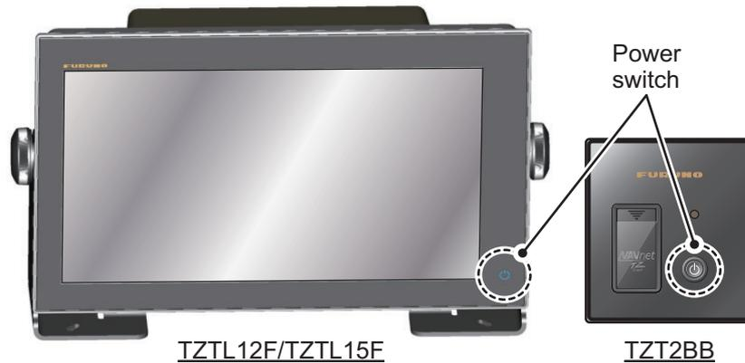
When you turn on the power, the equipment beeps twice and the start-up screen appears. After the startup process is completed, the [NAVIGATION WARNING] screen appears. Read the warning, then tap [OK]. Then, the last-used display appears.
