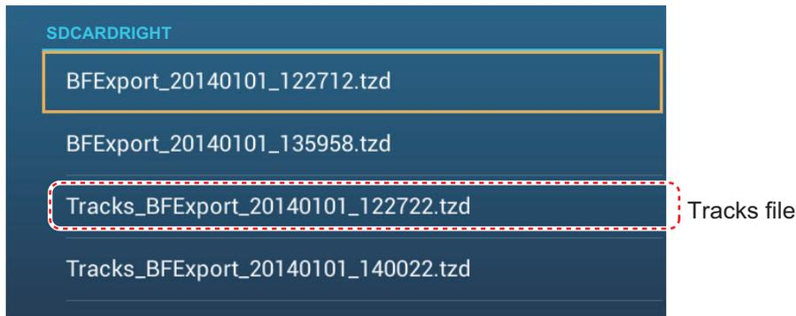
3. Tap [SDCardRight] (or [SD CardLeft]) on the SD card unit, [External] for USB port, or [Power Switch Left] (or [Right]) for Switch Box PSD-003. You are asked if you are sure to export points and routes.
