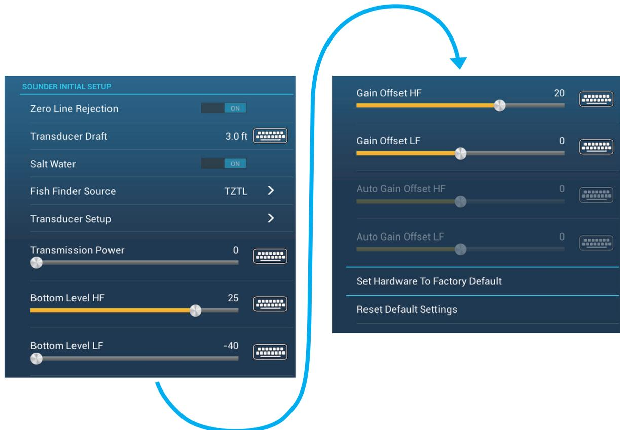
**[Zero Line Rejection]:** Turn the zero line (transmission line) on or off. When turned on, the transmission line disappears, which allows you to better watch fish echoes near the surface. The length of the transmission line changes with transducer used and installation characteristics.
