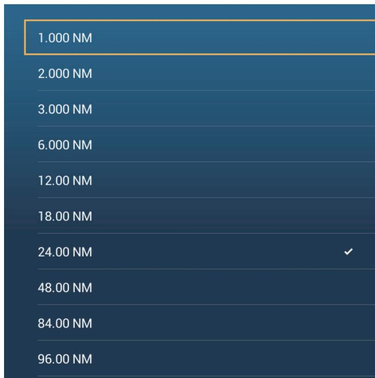
3. Tap a distance. Targets at a distance greater than selected here are not shown on the screen.
