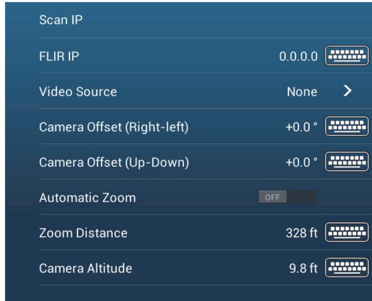
**Note:** To use the PTZ function of the FLIR camera with the NavNet TZtouch2, a setting (Nexus CGI Interface, port: 8090) is required at the FLIR camera. See the operator's manual of the FLIR camera for details.
